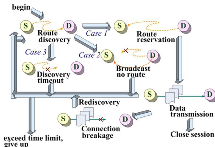
Figure 2-7: Overview of the on-demand routing algorithm.
