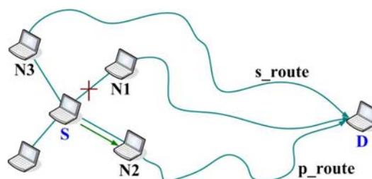
Figure 2-6: Rerouting when the path broken.
