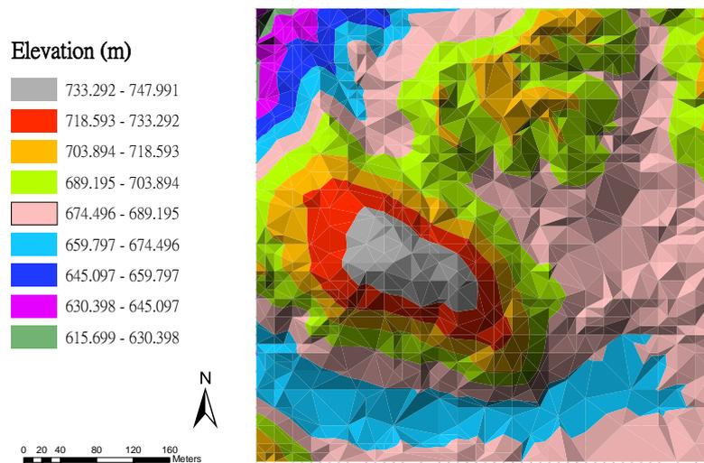
Figure 1. The TIN model of the FDP site
